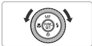
Turning the control dial allows you to perform operations such as choosing items or switching images. Except for a few operations, the same operations are possible with the buttons.
