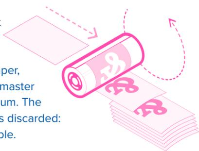
The drums rotate as paper is passed through the machine, making a print impression on each sheet. A two colour print means an impression from drum 1 first, then drum 2 second.
